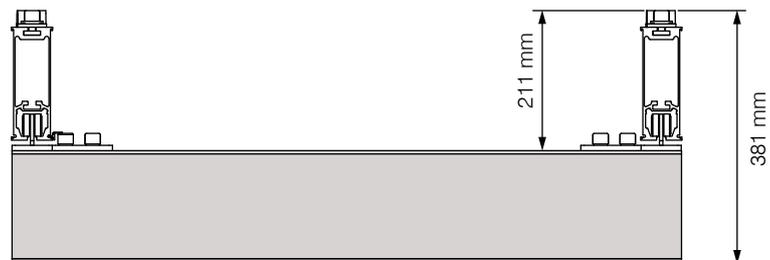
The rails can be cut to size so that room-covering and single track systems can be combined, even though different rail types are used in the two systems.
