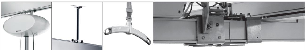
All Guldmann's hoist types lift with the help of a battery-driven motor and run in the rail system with the help of a travelling trolley, which is manually controlled or controlled with the help of a motor.
